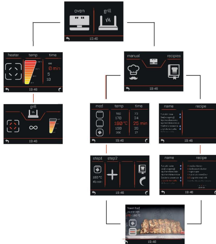
Figure 4.15. Full representation of info screens and GUI in the electric oven project with a grade of 3 (Team 4)
