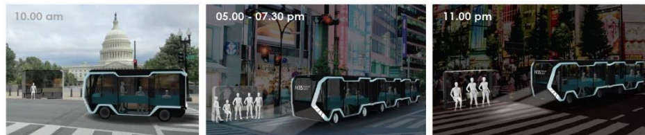
The number of modules are adjusted between 1 and 3 according to rush hours.
