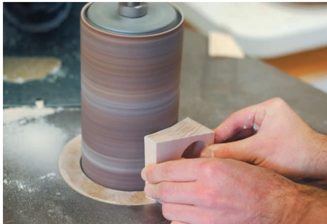
Figure 2.11. Finishing wood on a sanding machine (Halgrimsson, 2012)
