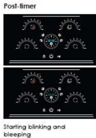
Figure 4.64. Partial representation of lights and minimal representation of sound in the vitroc ceramic cooktop project with a grade of 3 for lights and a grade of 1 for sound (Team 2)
