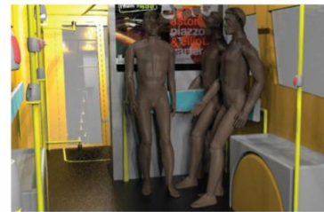
There are leaning units in the middle section of the bus for the passengers who get on the bus with a group.
