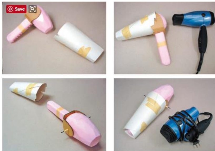
Figure 2.8. Low fidelity physical model of a hair dryer, made from foam and paper (Halgrimsson, 2012)
