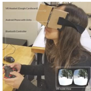
Figure 3.39. VR system consisting of the Google Cardboard, an Android smartphone running Unity's VR extension, and a Bluetooth controller (Chang, 2017)
