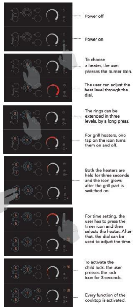
Figure 4.62. Partial representation of usage scenario (operating steps) in the vitroc ceramic cooktop project with a grade of 3 (Team 4)
