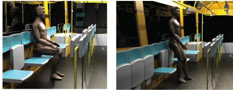
The seating units can be converted into a reclining unit upon request. In that way passenger capacity is increased.
